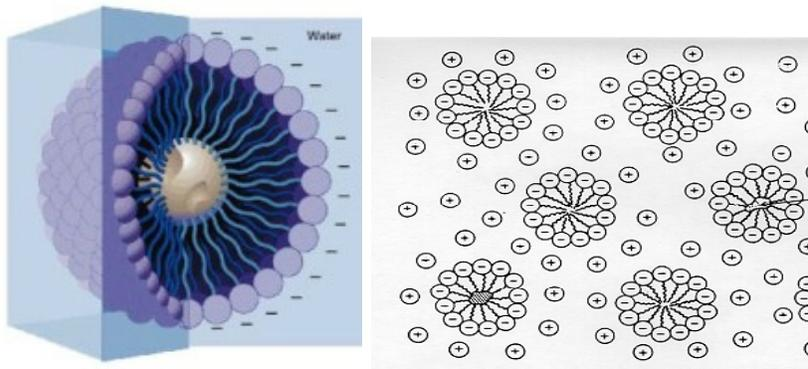
The head of the micelle is hydrophilic, meaning it likes water, while the interior portion is hydrophobic, meaning it avoids water. This provides a way to dissolve molecules that do not like water, in water.
